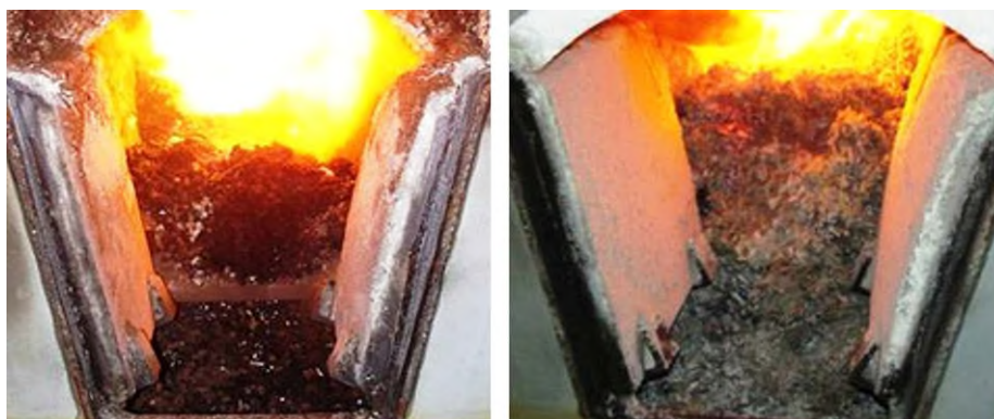
Fig. 2. View into the combustion trough: burnt-out ash of digestate 1 (left) and digestate 2 (right).
