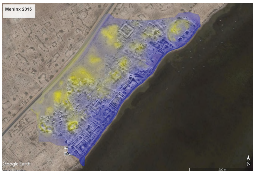
Fig. 8. Meninx, satellite image overlaid by the contour map and by the interpretation of the magnetometer data. The yellow parts mark the sectors with hills of debris; the blue are flat areas with distinct archaeological features.
