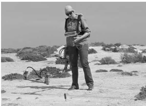
Fig. 4. Magnetometer prospecting at Meninx with the hand-held “duo-sensor” cesium magnetometer (J. Fassbinder).
