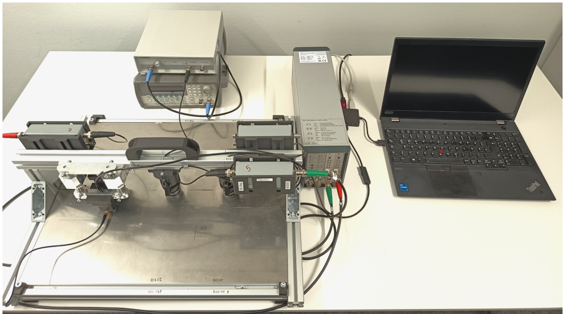
Figure 3.9: Top: Illustration of the verification setup with the arbitrary waveform generator, amplifier, AMSY-MB2-V1, and laptop [137, 138]. Bottom: Actual photograph of the mobile verification device. Adapted from [23].
