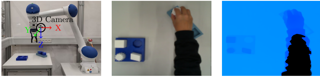
Fig. 8.1: Overview of the demonstration setup and recorded RGB-D data (a) Demonstration setup; (b) Color image; (c) Aligned depth image Adapted from Lu et al. (2025), licensed under CC BY 4.0.
