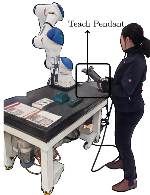
Fig. 2.7: Illustration of online robot programming with a Teach Pendant
