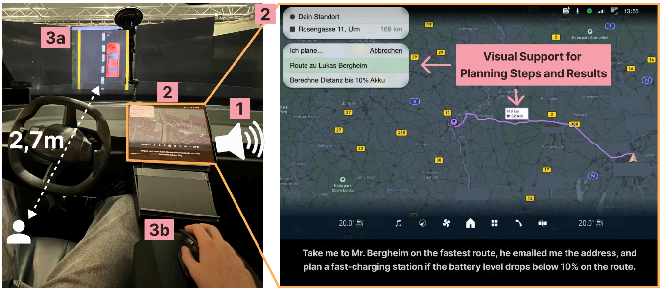
Figure 2: Study apparatus: 1. Speaker (Voice User Interface), 2. Center Display (Graphical User Interface), 3a. Driving simulation in the form of a lane-keeping task, 3b: mouse to correct continuous lateral drift for driving simulation.
