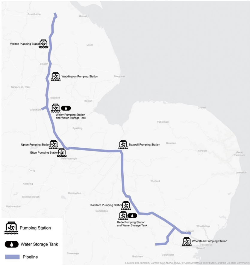
Fig. 5.1 Map of the Anglian Waters Strategic Pipeline project. Source: Author’s own representation according to Anglian Water, 2024
