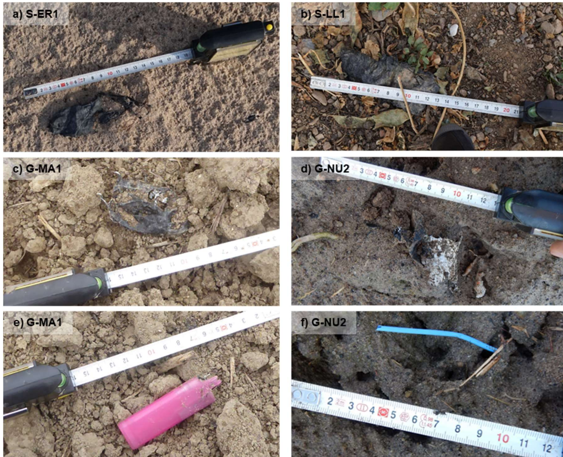
Figure 3.3: Photos a) S-ER1, b) S-LL1, c) G-MA1, and d) G-NU2 are from mulch film residues, while e) G-MA1 and f) G-NU2 are from residues from different sources. For abbreviations, see Table 3.1.
