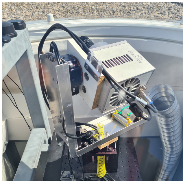
Figure 1. Photo of the scanning FAIM instrument. The azimuth rotation stage is below the horizontal metal frame, the second stage is vertically oriented to provide the possibility to rotate the camera to different zenith angles. The construction is counterweighted to prevent for unilateral strain and provide a longer lifetime of the mechanical components. The instrument is located below an air-ventilated acrylic dome at Oberpfaffenhofen.
