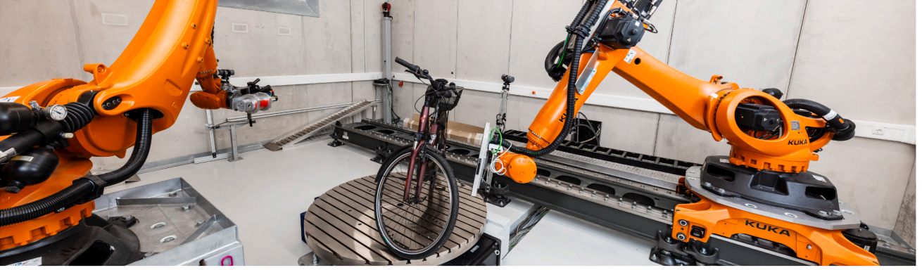
Fig. 2. The physical twin-robot CT system, featuring a bicycle to demonstrate system scale and a representative application.
