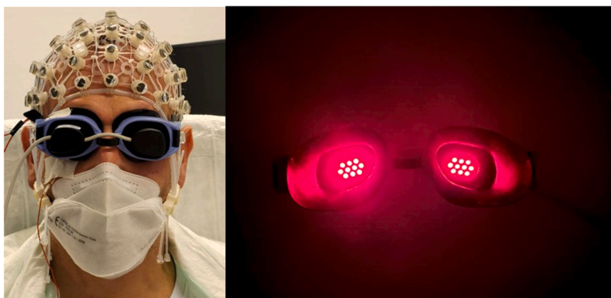
Fig. 1. Healthy participant with goggles delivering visual flicker, photodiode and 64-channel electroencephalography (EEG) system (left). Inside of the goggles with 10 red LEDs per eye (right).
