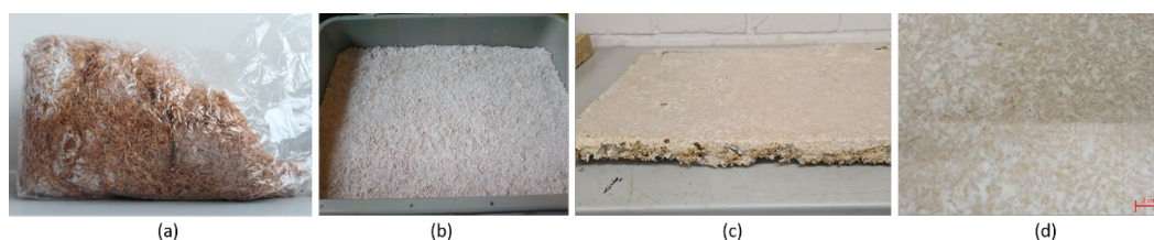
Figure 1. Mycelium cultivation and growth. (a) Inoculation of substrate using mycelium in growth bag; (b) growth of the material in a polypropylene (PP) growth box; (c) living mycelium after approximately 14 days of growth. (d) Zoom of the mature mycelium and the growth structure.
