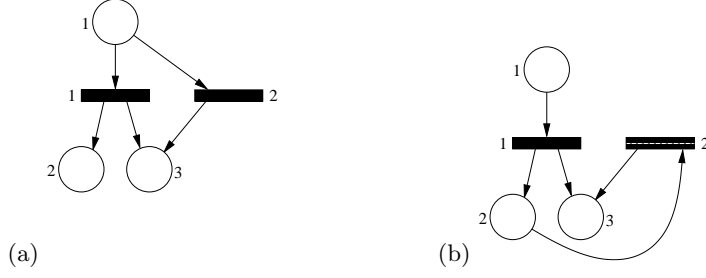
Fig. 8. Case 25 - p' = ((p_1, p_2), (p_1, p_3)) . p_1 has to be an element of the preset of the first contracted transition ( t_1 ), p_2 and p_3 have to be elements of the postset. To obtain p' , p_1 has to be element of \bullet t_2 and p_2 or p_3 have to be element of t_2^\bullet (a) leading to a circle when contracting in reverse order. Alternatively, p_2 can be element of \bullet t_2 and p_3 element of t_2^\bullet (b) leading to an arc with weight 2 when contracting in reverse order.
