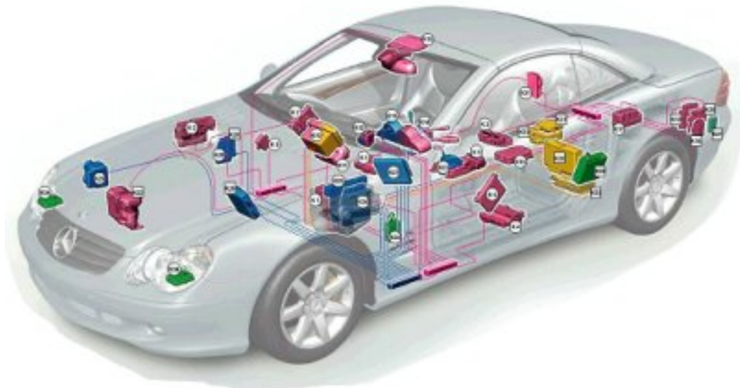
Figure 1.1.: Interconnected electronic control units in a modern vehicle [5]
