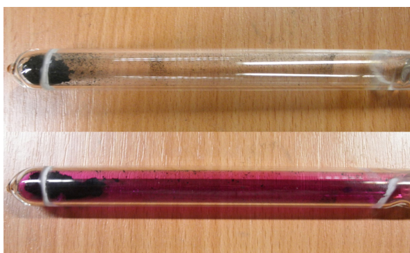
Figure 4.3: Top: closed evacuated quartz tube containing SWCNTs and iodine powders. bottom: Heated tube with violet iodine vapour
