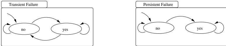
Fig. 7. Failure automata for transient and persistent failures
