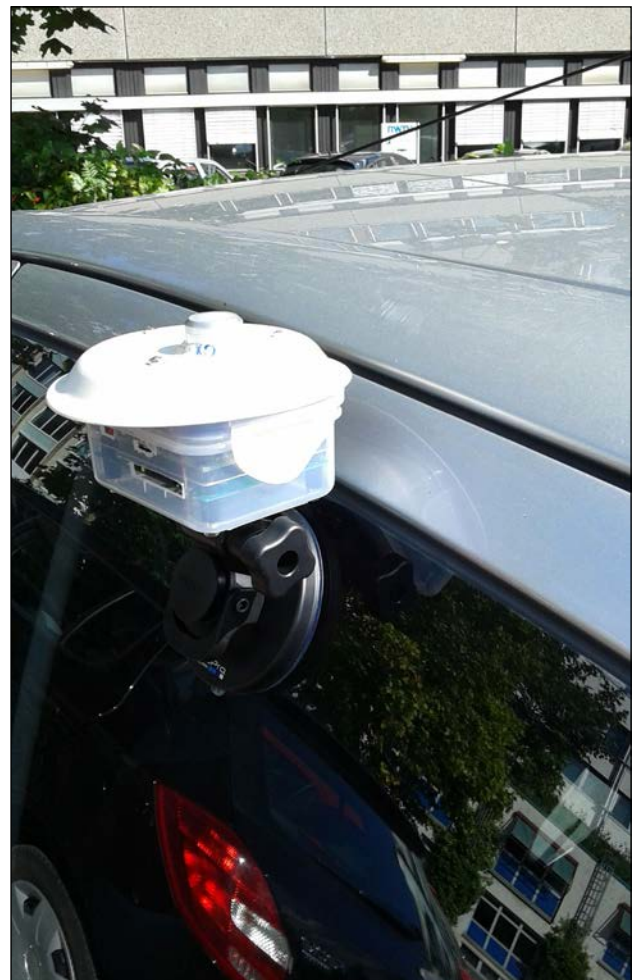
Fig. 5 Urbmobi 2.0 sensor installed on a car
