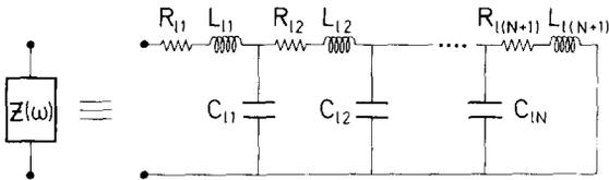
Fig. 5. Resistive transmission line model for the impedance  $Z(\omega)$ .
