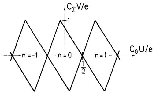
Fig. 3. The blockade diagram of a single-electron transistor with  $2C_2 = 10C_G = C_1$ . The capacitance  $C_\Sigma$  is the total capacitance of the island:  $C_\Sigma = C_1 + C_2 + C_G$ . The transistor conducts only outside the rhombic-shaped regions. Inside these regions, there is a constant number  $n$  of electrons on the island.
