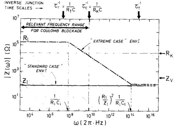
Fig. 6. Schematic behavior of the modulus  $|Z(\omega)|$  of the environment impedance, as a function of the frequency  $\omega$ . We have shown for comparison (i) the inverse junction time scales on the frequency axis and (ii) the resistance quantum  $R_k = h/e^2$  and the impedance of the vacuum  $Z_v = \sqrt{\mu_0/\epsilon_0}$  on the resistance axis.
