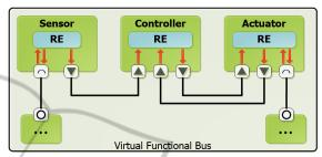
Figure 1: This simplified version of a typical sensor-actor system is an example of a structural AUTOSAR model without timing constraints. The arrows and the small black-and-white boxes indicate the communication direction between the REs.
