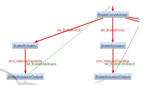
Figure 5: This cropped screenshot shows the results after the first run of the analysis. The dependencies' (graphs') colors indicate the respective dependency type whereas the annotated text shows the affected variables' names. Red lines point to problematic cycles that need to be fixed manually by the software engineer.
