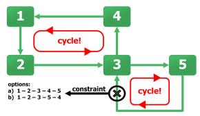
Figure 2: This figure shows a conflict example where the calculated output from "REI 3" is a necessary input for the calculation of "REI 5" and vice versa. This cycle has to be broken up via a constraint that allows the transferred data to be as old as one computing cycle or that imposes an execution order on the involved REIs (see Section 3.2).
