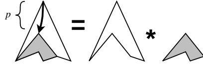
Fig. 7. Unfolding the tree abstraction, formally \mathbf{tree}(t, ino) = \mathbf{tree}|_p(t, ino, ino') * \mathbf{tree}(t[p], ino')
