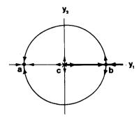
Fig. 1. Fixpoints of the noiseless motion in the rotating frame of reference: a stable, c unstable, b hyperbolic.
