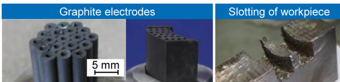
Fig. 39. Blasting erosion arc machining (BEAM) using bundled graphite electrodes for rough machining of blisk slots. Based on [227].
