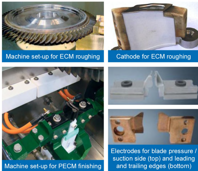
Fig. 20. Machine set-up and electrode design for DC-ECM roughing and PECM finishing of blisk geometries. Based on [55,152].
