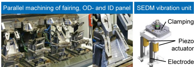
Fig. 40. Simultaneous machining of several seal slots in one set-up and schematic of twin piezo graphite electrode unit for vibration assisted EDM machining with standard interface. Based on [138,192].
