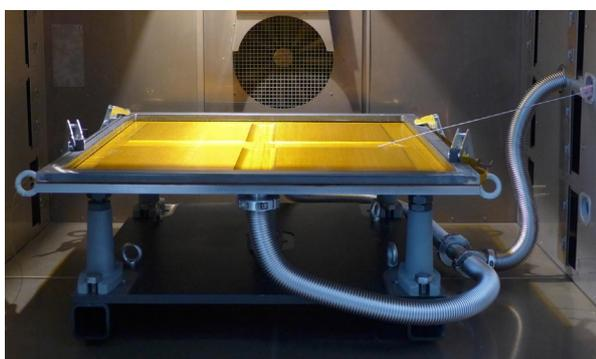
Figure 4 Transportable tooling (1 m × 1 m) for vacuum consolidation
