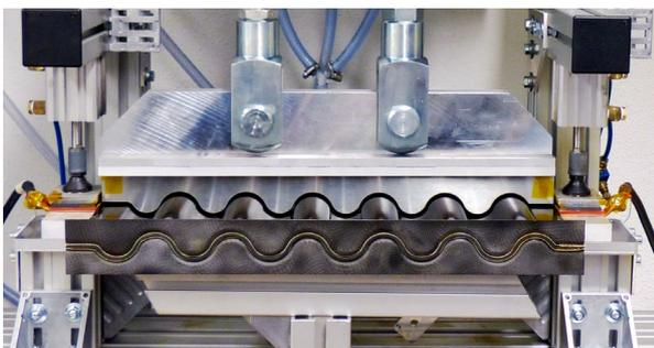
**Figure 11** Experimental setup for the implant resistance welding of the sine wave beam parts
