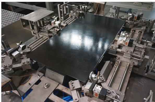
Figure 9 Clamping frame with 3D part after press process
