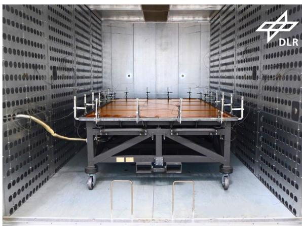
Figure 5 Movable tooling (2 m × 3 m) for vacuum consolidation
