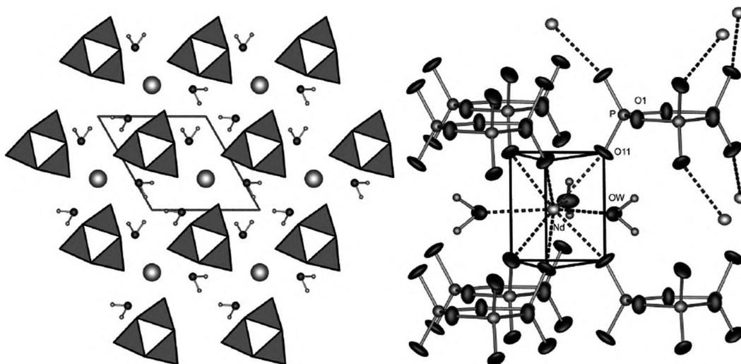
**Figure 1.** Crystal structure viewed along [001] and coordination of the neodymium atoms in  $\text{Nd}(\text{P}_3\text{O}_9)\cdot 3\text{H}_2\text{O}$ , the displacement ellipsoids are drawn on a probability level of 50%.
