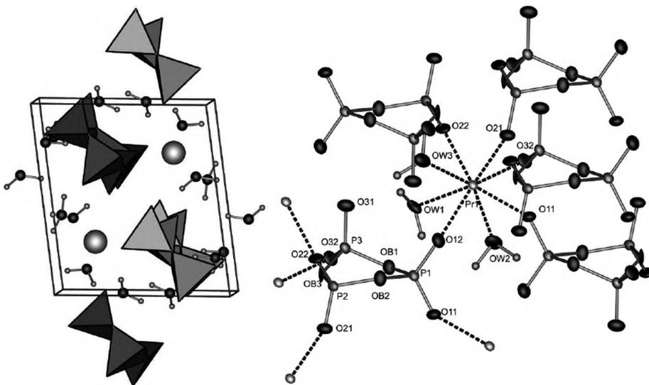
**Figure 4.** Crystal structure viewed along [100] and coordination of the praseodymium atoms in  $\text{Pr}(\text{P}_3\text{O}_9)\cdot 5\text{H}_2\text{O}$ , the displacement ellipsoids are drawn on a probability level of 50%.
