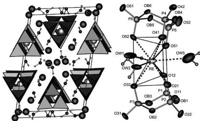
**Figure 5.** Crystal structure viewed along  $[010]$  and coordination of the praseodymium atoms in  $\text{Na}_3\text{Pr}(\text{P}_3\text{O}_9)_2 \cdot 6\text{H}_2\text{O}$ , the displacement ellipsoids are drawn on a probability level of 50%.
