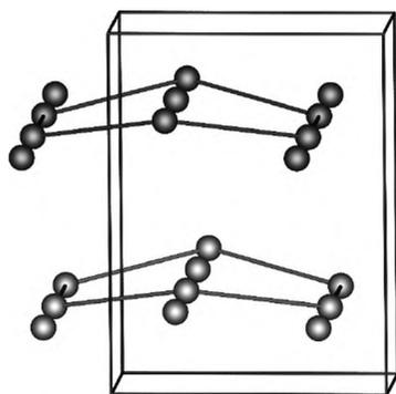
**Figure 6.** Representation of the distorted *hcp* type arrangement of the  $\text{RE}$  ions in  $\text{Na}_3\text{RE}(\text{P}_3\text{O}_9)_2 \cdot 6\text{H}_2\text{O}$  viewed along  $[100]$  ( $[001]$  running up); the differently greyed  $\text{RE}$  ions illustrate the two different layers, the lines between them the six-rings typical for densest packed layers.
