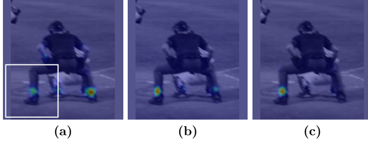
Figure 2.4: CPM estimate of the left ankle after stages 1 - 3. Output heatmaps are superimposed on the input image for easier interpretation. (a) Limited receptive field (white rectangle) of stage 1 leads to activations on both ankles. (b), (c) Additional spatial context in subsequent stages helps to uniquely identify the left ankle.
