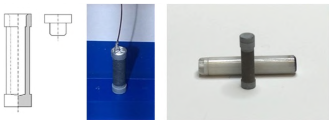
Fig. 1. Boron nitride insert used for the conductive heating: left: schematics; middle: insert after deposition of a thin Pt layer using physical vapor deposition. The contacting for the subsequent galvanization process is shown; right: final insert together with 4 mm spinner.
