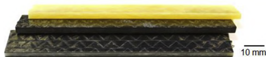
Fig. 1. Investigated SMC materials. From top to bottom: discontinuous glass fibre SMC (Dico SMC), continuous carbon fibre SMC (Co SMC) and hybrid continuous-discontinuous glass/carbon fibre SMC (CoDico SMC).
