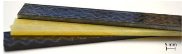
Fig. 3. From bottom to top: specimens made of continuous carbon fibre SMC, discontinuous glass fibre SMC and continuous-discontinuous hybrid glass/carbon fibre SMC.
