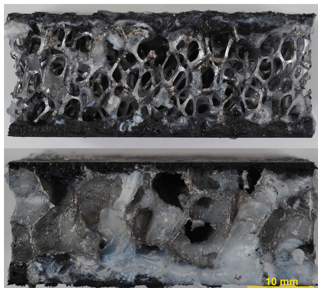
Fig. 4. Sandwich specimens with open (top) and closed cell aluminum core layer (bottom) directly after 240 h of exposure to the corrosive environment.
