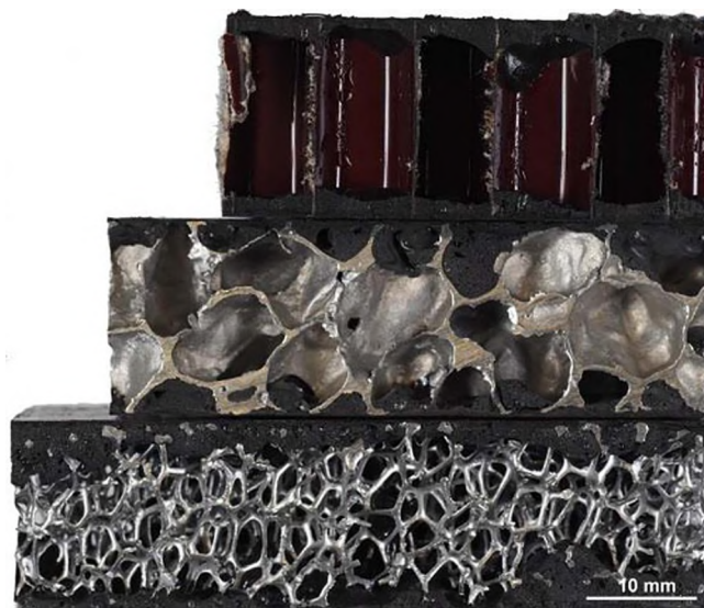
Fig. 1. Sandwich specimens with Nomex honeycomb core (top), closed cell (middle) and open cell aluminum foam core (bottom).
