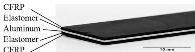
Fig. 1. FMEL specimen with CFRP face layers, aluminum core and elastomer interlayer.
