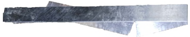
Fig. 14. FML fatigue specimen loaded at 25% of UTS showing delamination and aluminum fractures.
