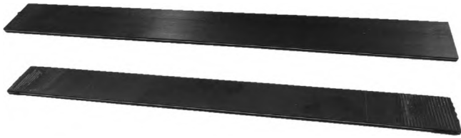
Fig. 5. The upper FMEL specimens was depicted before and the lower specimen after fatigue loading.
