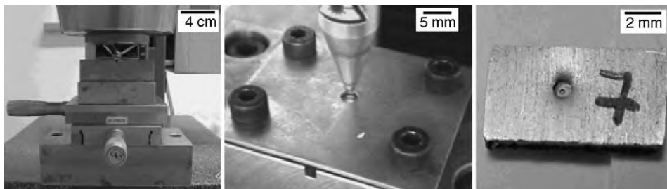
Fig. 2. Experimental setup for the push-out-tests: hardness probe with indenter (left), positioning with a light pointer (centre), specimen with wire pushed out (right).
