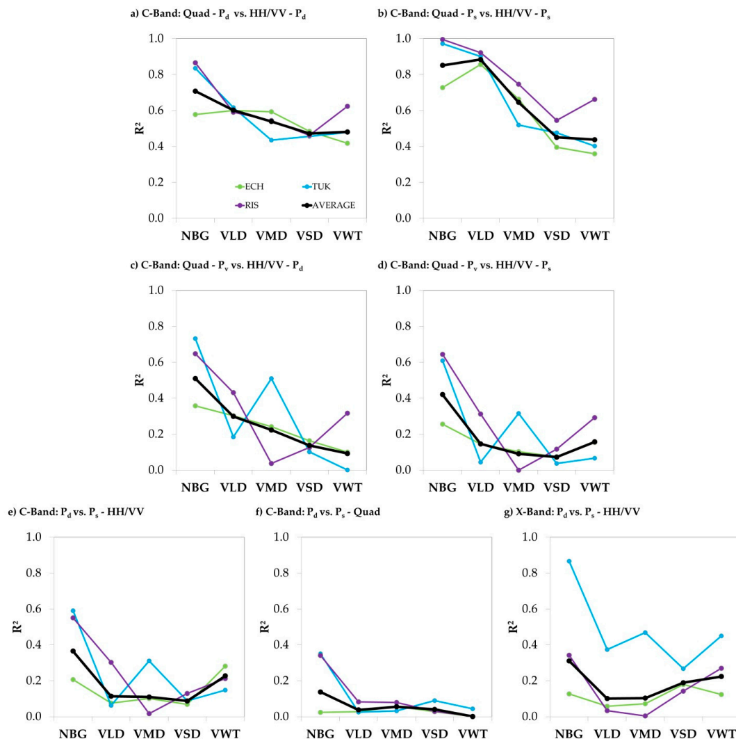
Figure 3. Squared linear Pearson correlation coefficients ( R^2 ) for none-water land cover classes (NBG, VLD, VMD, VSD, VWT) of: (a) double bounce ( P_d ) of the two and three component decomposition; (b) surface scattering ( P_s ) of the two and three component decomposition; (c) volume scattering ( P_v ) of three and P_d of the two component decomposition (C-Band); (d) P_v of three and P_s of the two component decomposition (C-Band); (e) P_d and P_s of the two component decomposition (C-Band); (f) P_d and P_s of the three component decomposition (C-Band) and (g) P_d and P_s of the two component decomposition (X-Band). Abbreviations of the test sites: TUK: Tuktoyaktuk, RIS: Richards Island, ECH: East Channel of the Mackenzie River.
