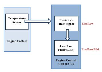
Fig. 2. Physical layout of an AUTOSAR compliant engine-coolant system function - Engine coolant temperature sensor connected to an ECU
