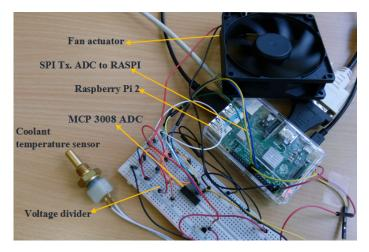
Fig. 5. Experimental set-up - Sensor interfacing to hardware
