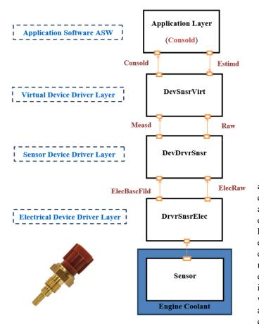
Fig. 3. AUTOSAR design pattern for a standard sensor
