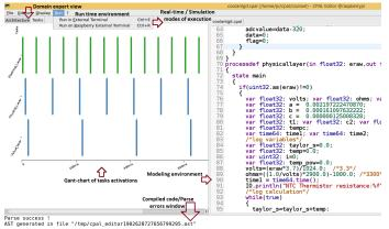
Fig. 4. An integrated environment, here the CPAL-Editor, with the code of the model, the Gantt chart of the processes activations and the possibility to execute the models in simulation and real-time mode both locally or on a target.
