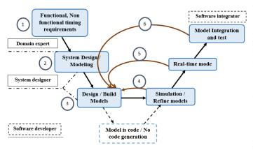
Fig. 7. Model interpreted engine function development flow - steps and stakeholders involved
