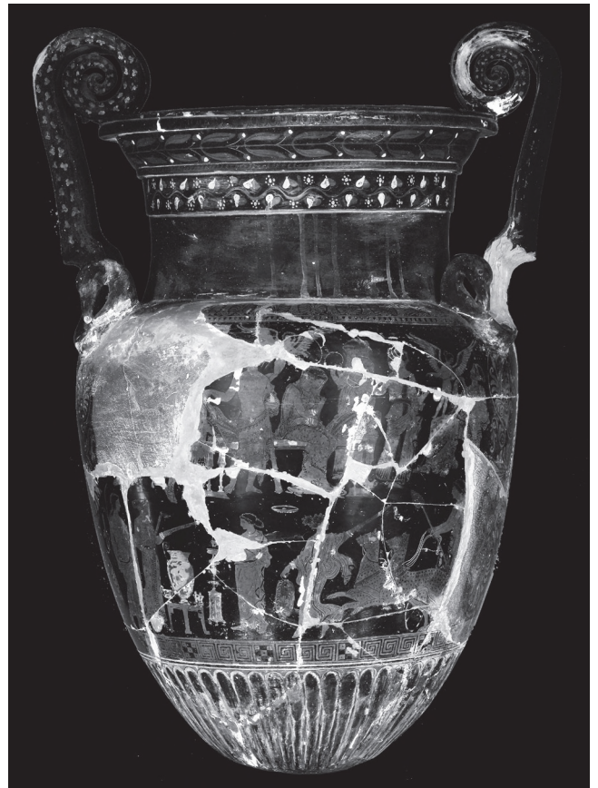
Fig. 9 UV image of krater (F 3257) showing fluorescence of 19 th century interventions.
