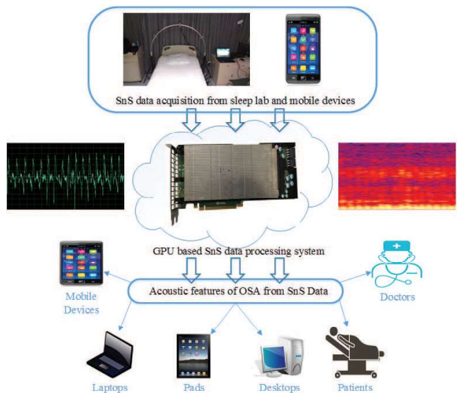
Fig. 1. The proposed GPU-based system for processing SnS data collected in the hospital or via personal smart devices.
