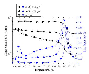
**Figure 7.** 3PB Temperature sweep at 1 Hz for all lay-ups with aluminum on the outside. The solid lines are fitted to the measurement steps every 2.5 °C from -70 °C to +200 °C and every 5 °C from -20 °C to 200 °C. For better visibility, only a few markers are displayed.
