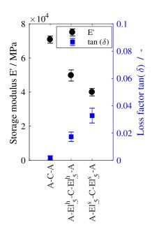
**Figure 8.** Storage module and loss factor for all specimens with aluminum on the outside at 20 °C and 1 Hz. Three specimens for each lay-up
