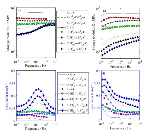
**Figure 10.** Master curves for all specimens at  $T_{Ref} = -40 \degree C$  (**a**,**c**) and  $T_{Ref} = 80 \degree C$  (**b**,**d**). For better visibility, fewer markers are displayed for the fitted curves.
