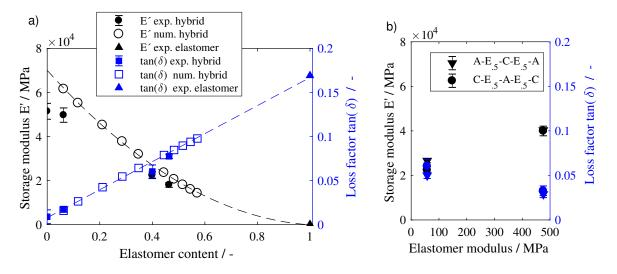
**Figure 13.** (a) Influence of elastomer content = (total thickness of both elastomer layers)/(thickness of specimen)) for a (C-El<sup>s</sup>-A-El<sup>s</sup>-C) lay-up; (b) experimental results for the influence of the elastomer modulus.
