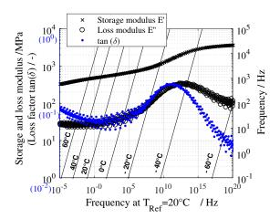
Figure 4. Master curve nomogram for tension DMA on the hard elastomer El<sup>h</sup><sub>5</sub>.
