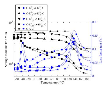
**Figure 5.** 3PB Temperature sweep at 1 Hz for all lay-ups with CFRP on the outside. The solid lines are fitted to the measurement steps every 2.5 °C from -70 °C to +200 °C and every 5 °C from -20 °C to 200 °C. For better visibility, only a few markers are displayed in addition to the fitted solid lines.
