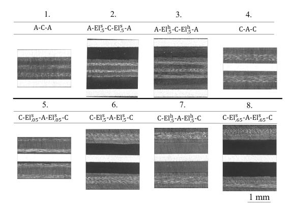
Figure 1. Micrographs of the FML and FMEL lay-ups listed in Table 2.
