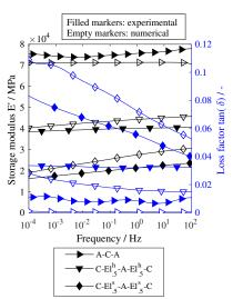
**Figure 12.** Experimentally and numerically determined master curves for a reverence temperature of 20 °C for selected lay-ups.
