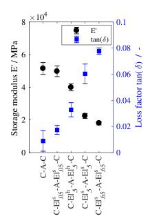
**Figure 6.** Storage module and loss factor for all specimens with CFRP on the outside at  $20 \degree C$  and 1 Hz. Three specimens for each lay-up.
