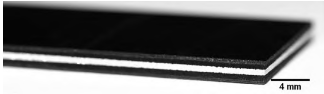
Fig. 1. FMEL specimen with CFRP face layers, elastomer interlayers and an aluminum core layer.
