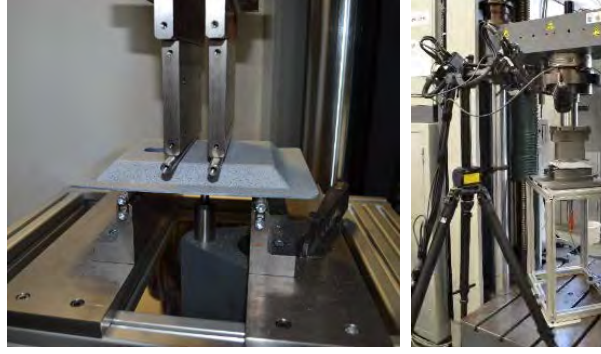
Fig. 3 Setup of four- point bending test with DIC measurement.
