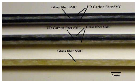
Fig. 1 CoDiCo Laminates: CGC (top), GCG (middle) and G (bottom)
