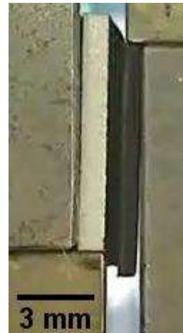
Fig. 2 FML with elastomer interlayer in the edge shear test
