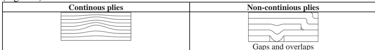
**Figure 7: Waves at continuous vs. non-continuous plies**
