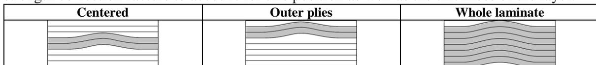
**Figure 8: Position of the wavy layers in the laminate**
