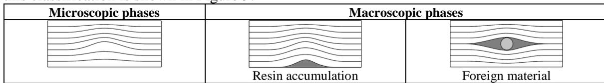
**Figure 9: Microscopic vs. macroscopic distributed phases in wavy regions**
