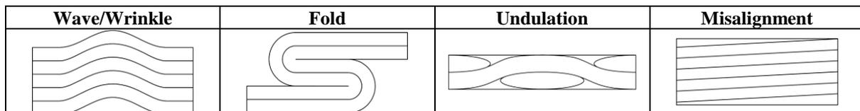
**Figure 1: General definition of deviations from the intended fiber orientation, i.e. wave/wrinkle, fold, undulation and misalignment.**
