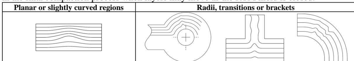
**Figure 11: Waves in flat or slightly curved areas vs. waves in radii, transitions or brackets**
