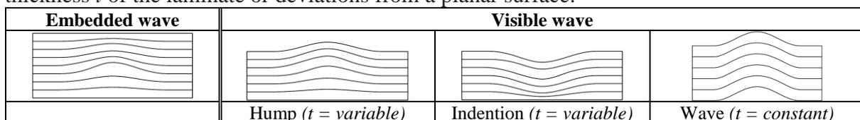
**Figure 5: Embedded vs. visible waves**
