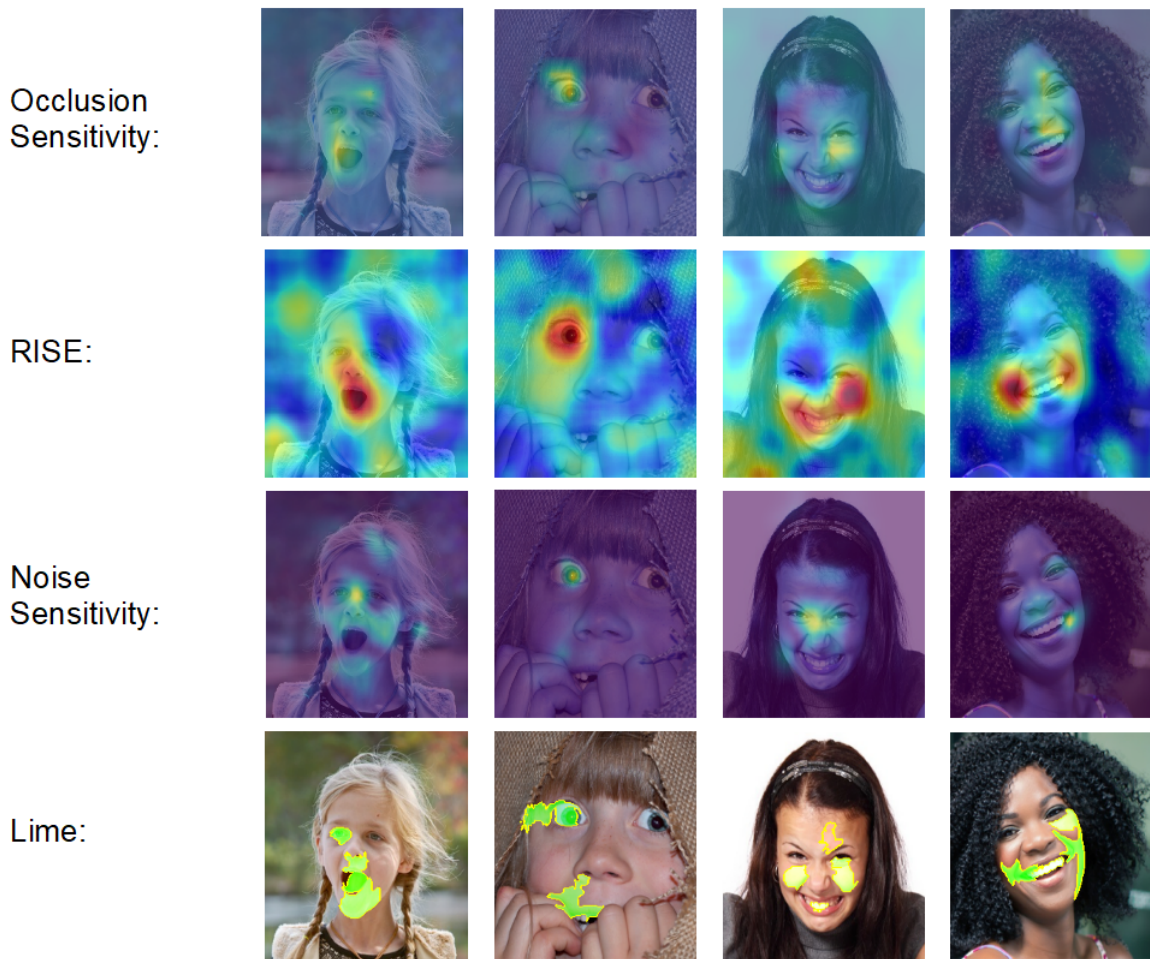
Figure 6.3: Explanations for different facial expressions, based on the previously described explanation approaches. The emotions from left to right being: surprise, fear, disgust, and happiness. As already mentioned, the third image was incorrectly classified as happy.
