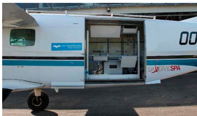
Figure 3. Cessna C208 carrying the SARSense radar setup. The top left and bottom right antennas are for L-band, the bottom left and top right antennas for C-band.
