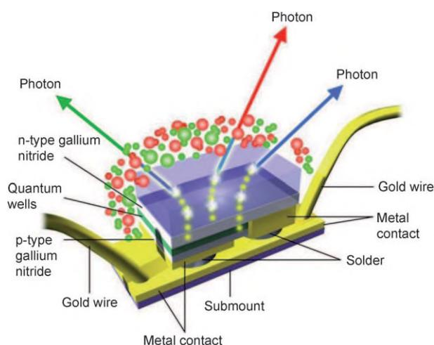
**Figure 2.** Schematic depiction of a warm-white-emitting diode<sup>[17]</sup> based on a blue LED coated with a green and a red phosphor.
