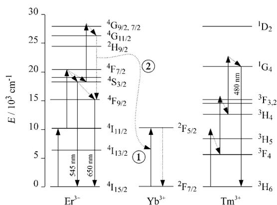
**Figure 10.** Upconversion mechanism in codoped  $\text{Yb}^{3+}/\text{Er}^{3+}$  and  $\text{Yb}^{3+}/\text{Tm}^{3+}$  compounds, respectively;  $\text{Yb}^{3+}$  is excited by infrared light (1) and transfers its energy onto an  $\text{Er}^{3+}$  ion, which then emits green or red light. Alternatively, the  $\text{Yb}^{3+}$  ion transfers its energy onto a  $\text{Tm}^{3+}$  ion, which emits blue light (illustration adapted from reference [129]).
