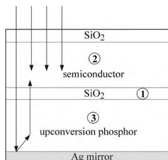
**Figure 8.** Principle of a solar cell; incident sunlight passes the semiconductor solar cell (2) coated with  $SiO_2$  (1) and the layer containing the upconversion phosphor (3) before being reflected on a silver mirror (illustration adapted from reference [126]).
