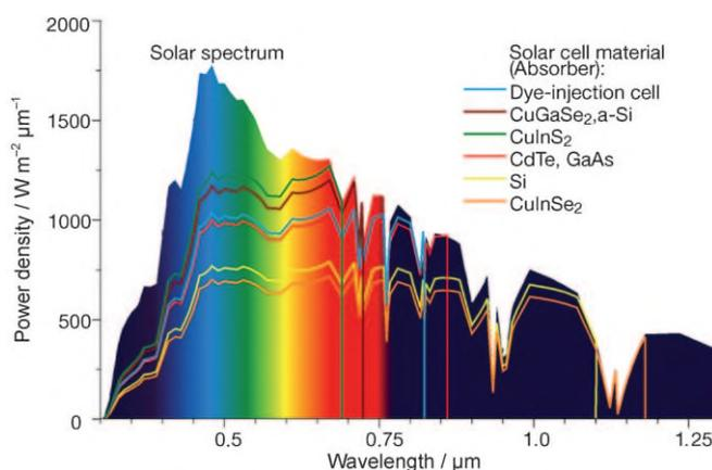
**Figure 7.** Solar emission spectrum as observed on the surface of the earth; the absorption lines of important semiconductors for use in solar cells are indicated.<sup>[113]</sup>
