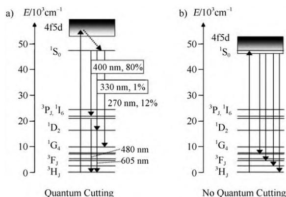
**Figure 6.** Illustration of the quantum-cutting process in  $\text{Pr}^{3+}$ -doped compounds<sup>[107]</sup> (left); if the  $4f5d$  levels are too low energetically, no quantum cutting can be observed (right).
