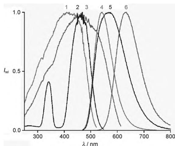
**Figure 3.** Excitation and emission spectra of phosphors for white LEDs;  $\text{SrSi}_2\text{O}_2\text{N}_2:\text{Eu}^{2+}$  (excitation: 1, emission: 4),  $\text{YAG}:\text{Ce}^{3+}$  (excitation: 2, emission: 5),  $\text{Sr}_2\text{Si}_5\text{N}_8:\text{Eu}^{2+}$  (excitation: 3, emission: 6).<sup>[17]</sup>
