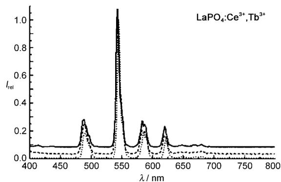
**Figure 5.** Emission spectra of  $\text{LaPO}_4:\text{Ce}, \text{Tb}$  under UV illumination (254 nm); as-prepared nanoparticles (----) and nanoparticles tempered for 30 min at  $650^\circ\text{C}$  (—) compared with the macroscale phosphor (.....; illustration adapted from reference [93]).
