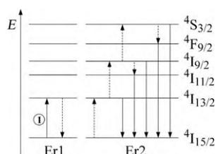
**Figure 9.** Upconversion process between two  $\text{Er}^{3+}$  ions; after excitation of an  $\text{Er}^{3+}$  ion (Er1) with 1520 nm (1), its relaxation may lead to a multiple energy transfer onto a second  $\text{Er}^{3+}$  ion (Er2), which subsequently emits light of shorter wavelength; dashed lines represent radiationless transitions (illustration adapted from reference [125]).
