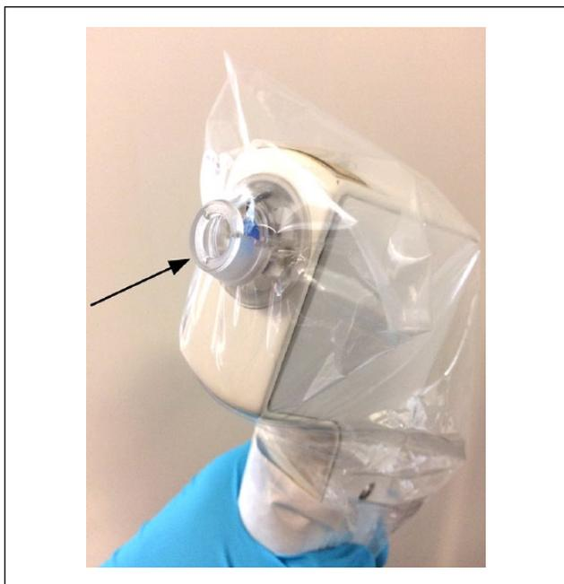
**Figure 1.** Optical coherence tomography probe, enclosed in sterile sheath over which is fitted a sterilized “standoff” (arrowed) to set skin at the correct focal distance.
