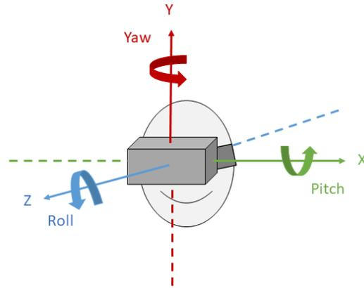
**Figure 4.4:** A coordinate system of 6 DOF. The position is listed as a set of x,y,z coordinates, where x is for left-right, y is for up-down, and z is for forward-back. Orientation is listed as a quaternion where the pitch is leaning forward or backward (rotation x-axis), yaw is rotating left, or right (rotation y-axis), and roll is bending left or right (rotation z-axis).
