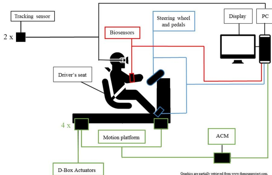
**Figure 4.1:** Concept of the VR driving simulation with an HMD operationalized in the experiments.
