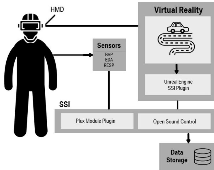
**Figure 5.3:** Architecture of the proposed approach showing the connection between the sensors and the virtual environment. RESP stands for respiratory sensor.
