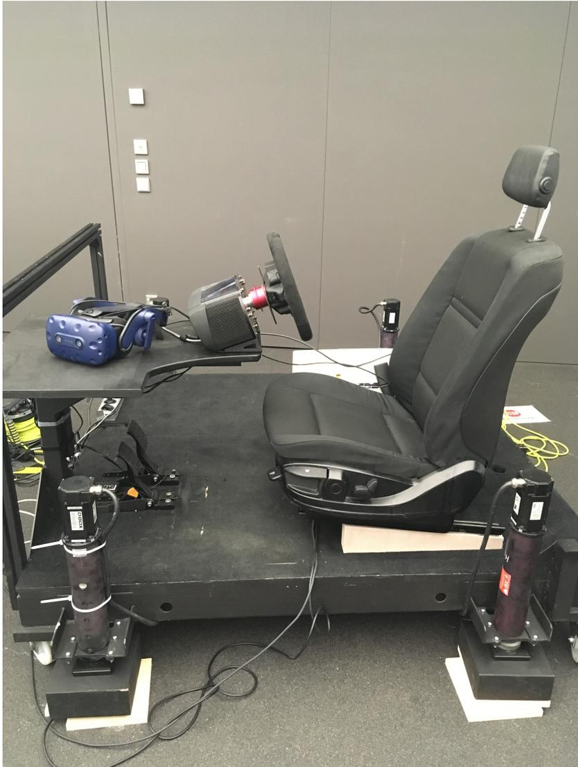
**Figure 4.2:** Setup of the VR driving simulation including the HMD (HTV Vive Pro), motion platform(D-Box), driving seat, steering wheel, and pedals (Fanatec).
