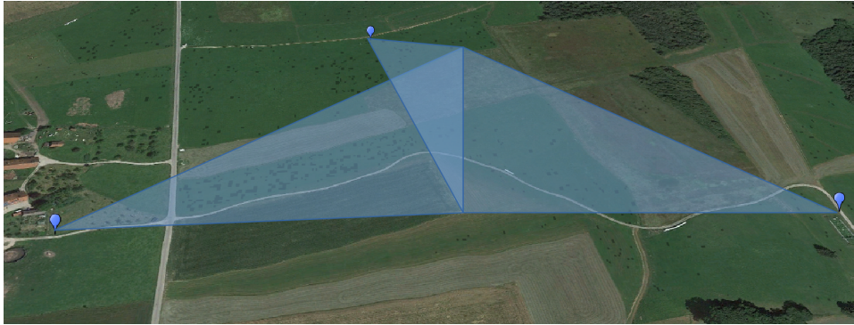
FIGURE 4.12: Structure of the VirtualTower installation. Three Lidar beams form a virtual tower at the common center of three intercepting beams.
