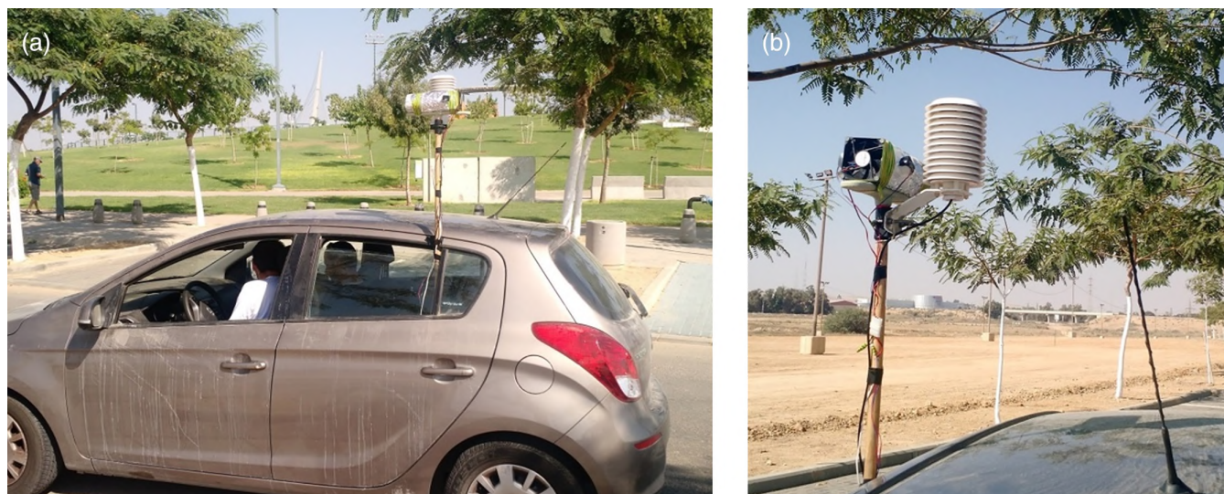
FIGURE 2 Two type T thermo-couples mounted on the rooftop of a car at about 2 m height (a) and the thermo-couples shielded in a mechanically aspirated 10 cm plastic tube (b)
