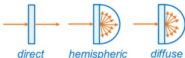
Figure 3. Measurement of direct, hemispheric and diffuse transmittance.
