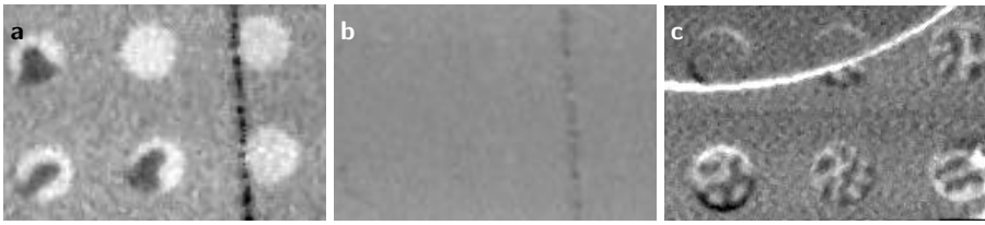
Figure 3.5 | Temperature effect in Co/Pt material Co/Pt 6 (a) STXM graph of another area of the same sample shown in Fig. 3.3a. The black line is the left border of the transmission line. (b) The same sample area after sending current pulses through the wire. The magnetic contrast has vanished completely. (c) Another area of the same sample. Here, only the material underneath the curved transmission line shows out-of-plane magnetic contrast, even in the disk that is partially covered by it.
