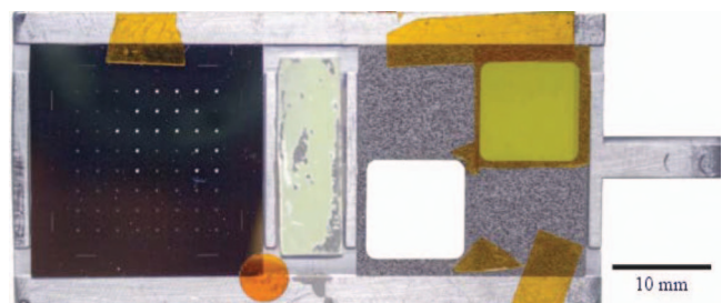
FIG. 5. Photograph of a sample holder with one multi-window sample (left), one adapter plate for smaller samples (right), and a fluorescence screen (center).
